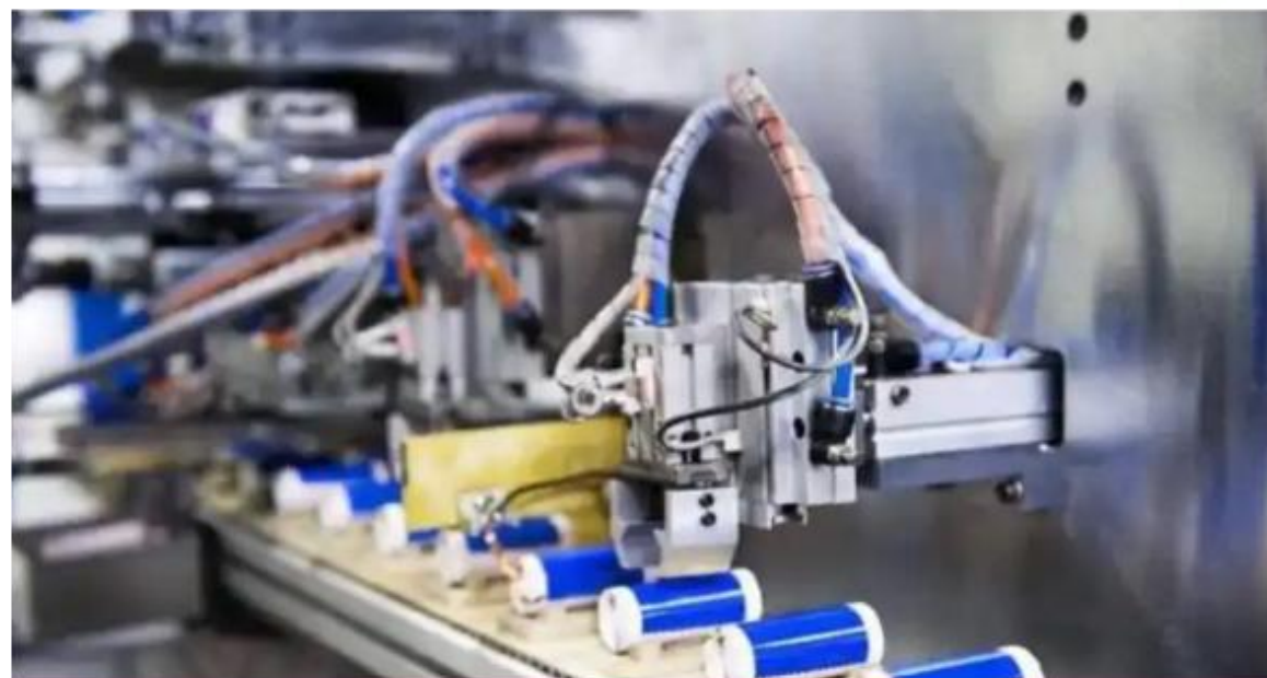
锂电制造 卷绕机 Lithium electric manufacturing winding machine
