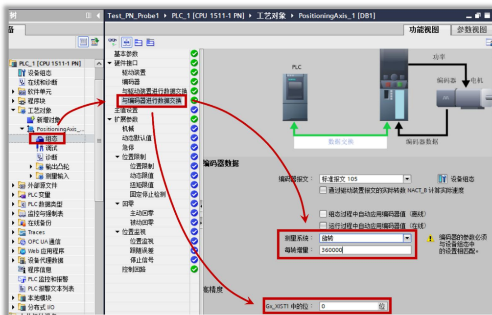
figure9-36 Settings for data exchange with the encoder when applying a rotating motor
