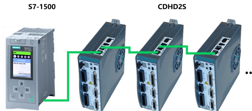
figure9-2 SERVOTRONIX CDHD2S-PN-RS with Siemens S7-1500 Hardware Topology
