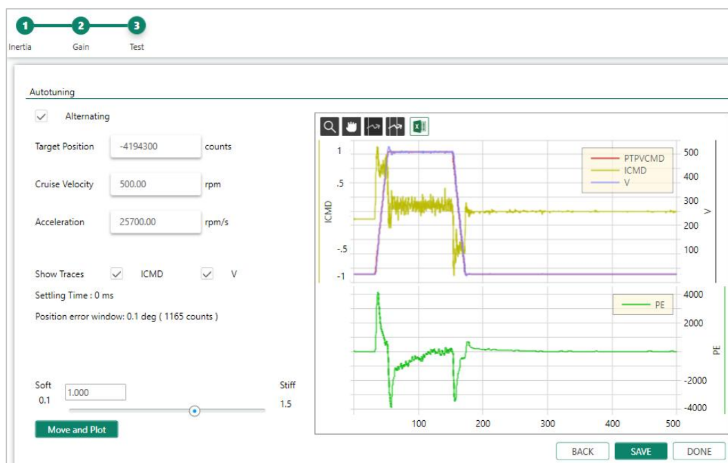
Figure 8-13 PC-based autotuning wizard – test movement quality
